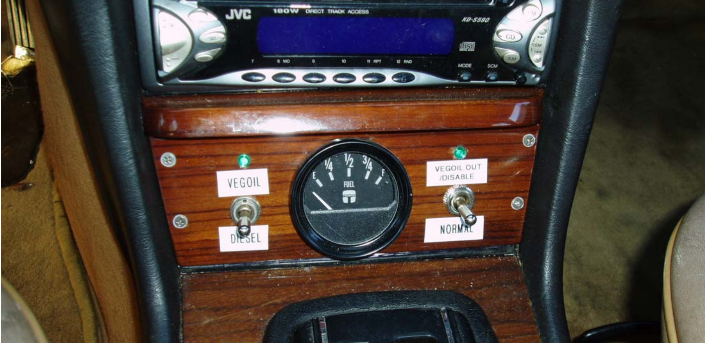
CONTROL PANEL INSTALLED AND LABELED
