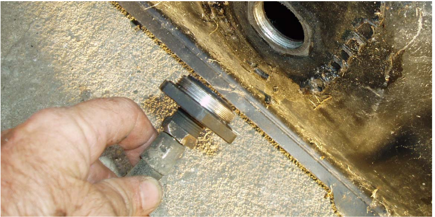
STRAINER CUT OFF ORIGINAL TANK OUTLET
