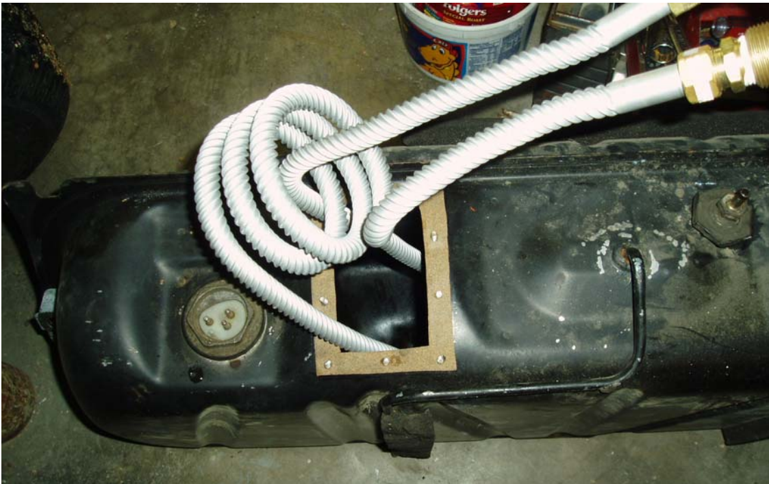
HOLE CUT IN TOP OF TANK. HOLES WERE THREADED AND MACHINE SCREWS INSERTED FROM INSIDE THE TANK. USE PAPER OR CORK GASKET. VEGOIL WILL ATTACK RUBBER
