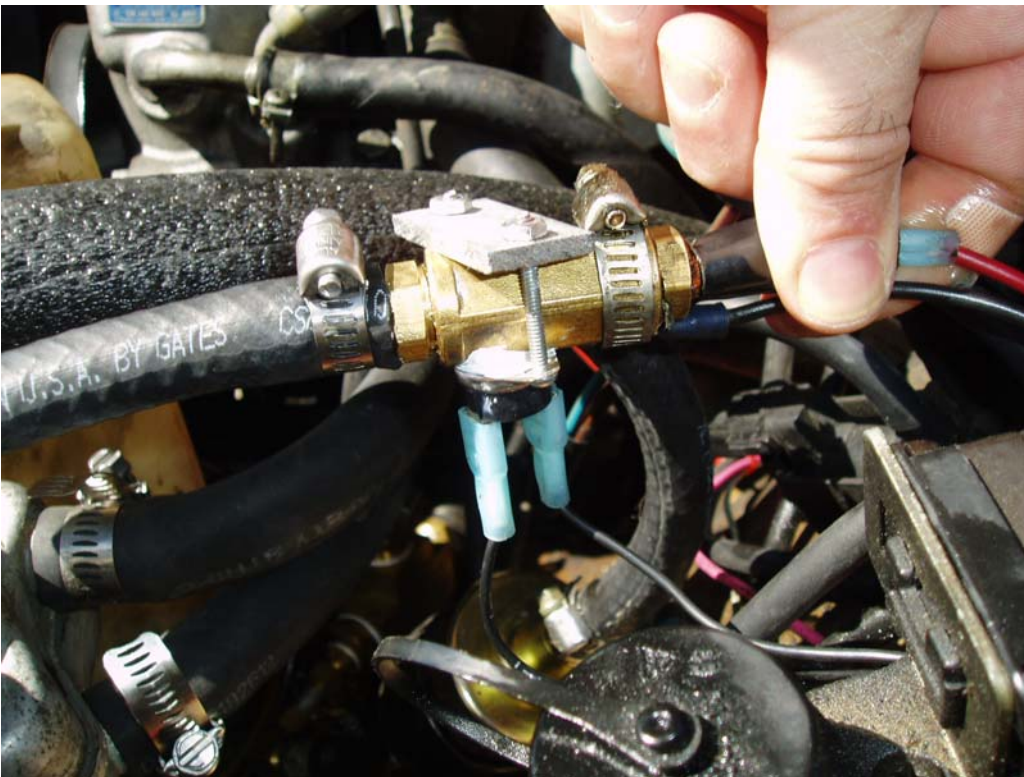
PLUMBING TO HEATED FILTER. GLOW PLUG LINE HEATER INSTALLED BEFORE FILTER. VEGOIL PUMP SHOWN BELOW GLOW PLUG HEATER.
