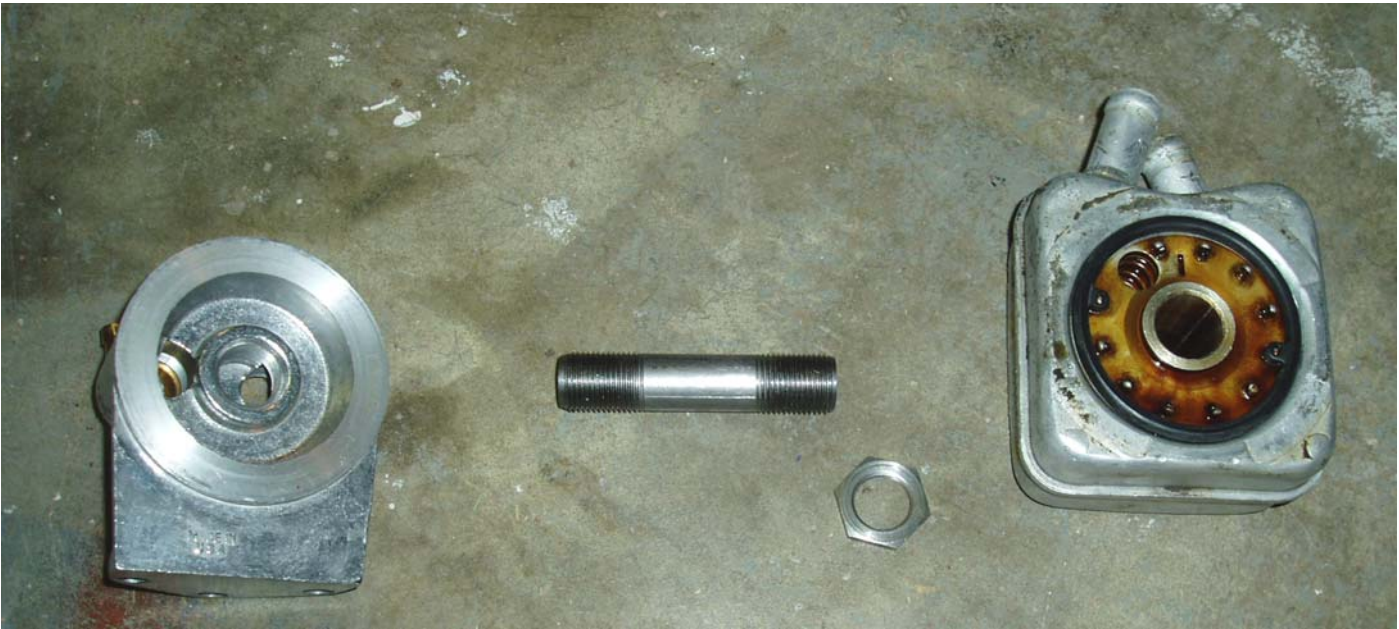
VW OIL COOLER FOR HEATED FILTER
