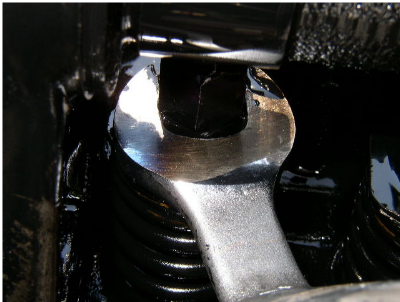
Valve adjusting wrench is on the lower lock nut ready to take tension off the top adjusting nut.
