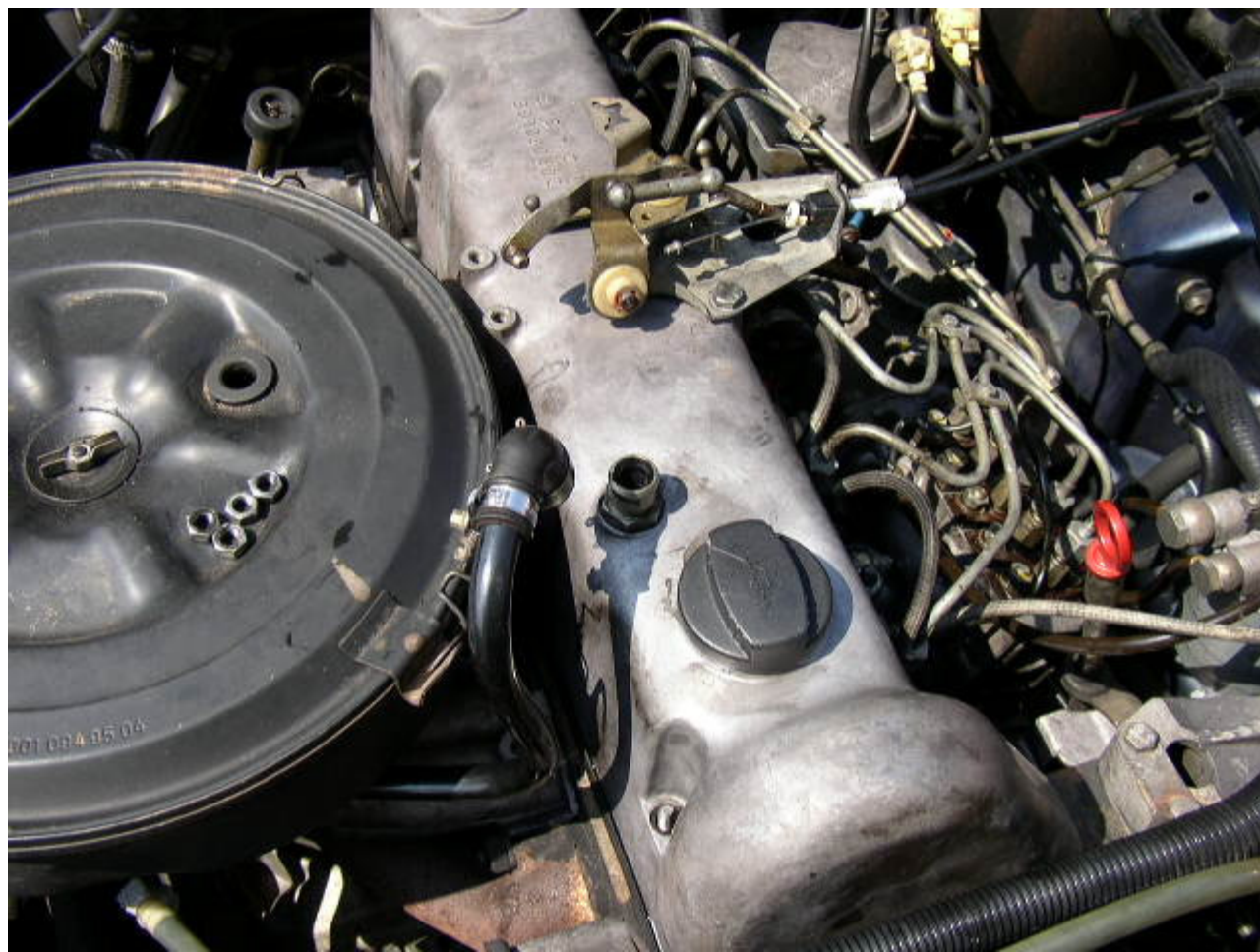
Valve cover back on and ready to be bolted down.
